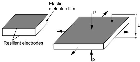
Figure 1: Simple working principle of an EAP
