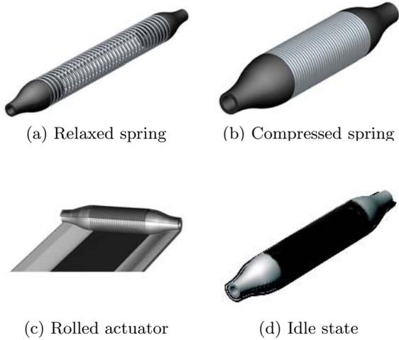
**Figure 6: Schematic of cylindric dielectric polymer actuator**
