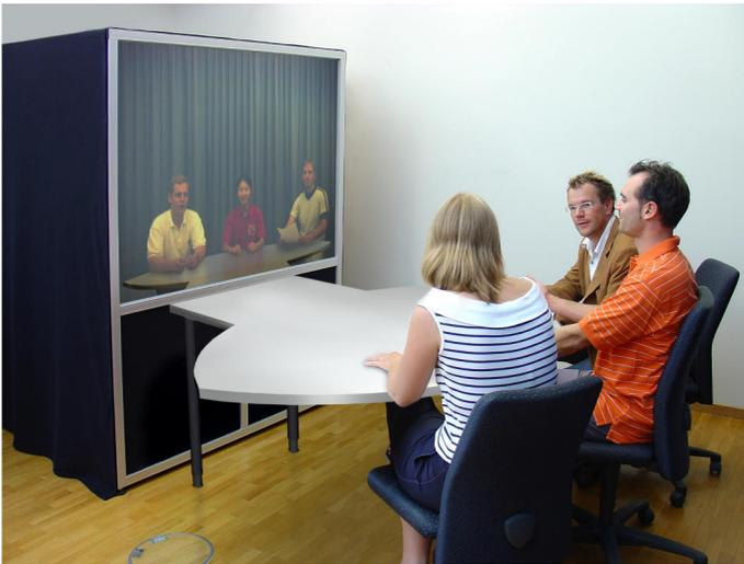
**Fig. 7.** The real table is extended by a virtual one, using a holographic projection screen
