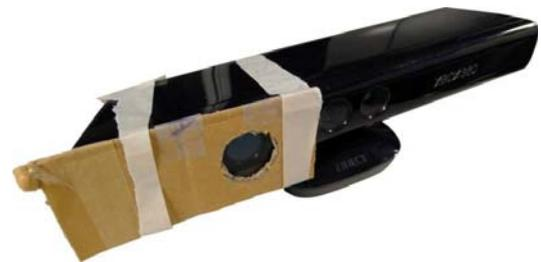
Figure 10: A linear polarization filter is used to attenuate the Kinect's IR-light. A piece of cardboard holds it in place.
