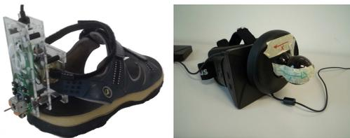
Figure 2: Electromagnetic tracking system and step sensor
