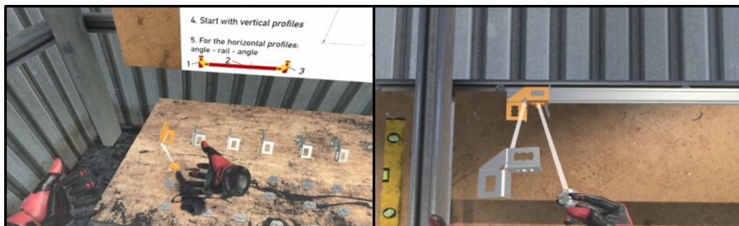
Fig. 5 Implemented AG methods - Highlight and in-situ line from center of FOV to target object (left). Target orientation indication and in-situ line from center of FOV to target position (right).
