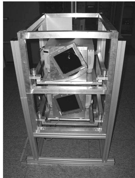
**Figure 4. Stereo projection rack with LC-shutters**
