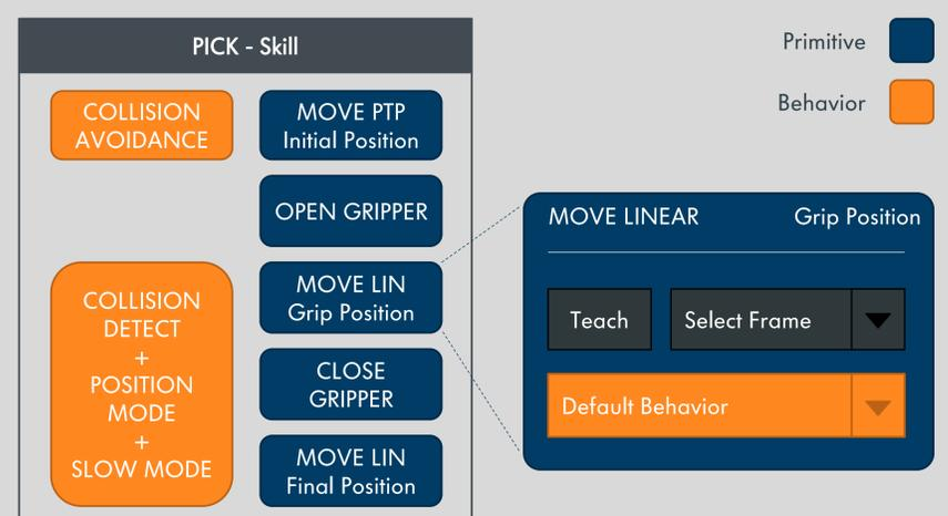
Fig 2: Definition of a pick-skill using primitives and behaviors.
